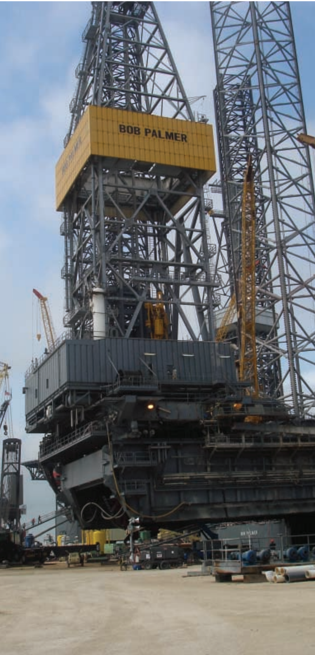
The Bob Palmer, a Gorilla-class jack-up rig (Photo courtesy of Jackie Reuss)
